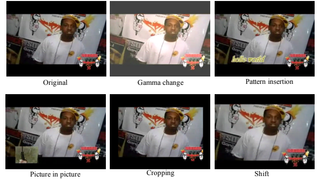
Figure 5. Samples of query videos with different transformations.
