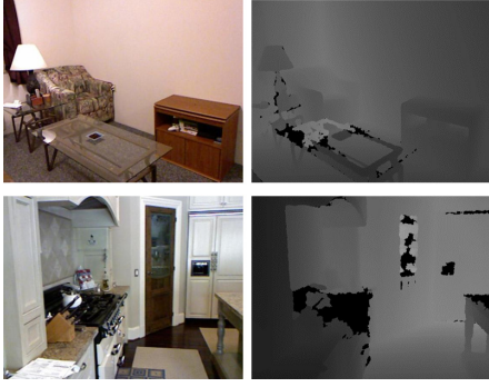
Figure 3: Sample images and their associated depth maps in the the SUNRGBD dataset.
