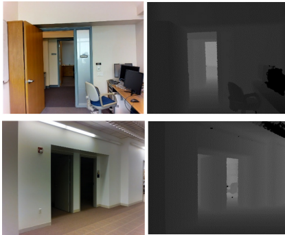
Figure 5: Sample images and their associated depth maps in the Stanford 2D-3D-S dataset.
